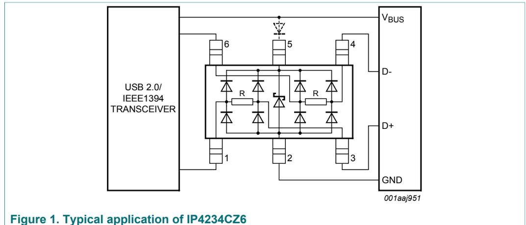
**Figure 1. Typical application of IP4234CZ6**
